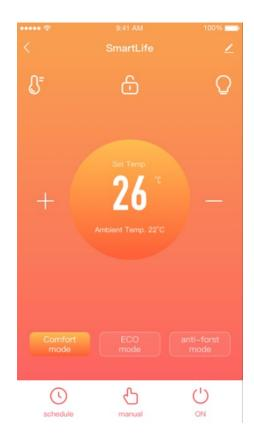
You can change the heater's mode by pressing the "mode" buttons. You can adjust the mode's temperature using the + and – buttons.
